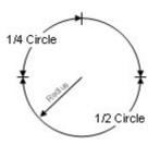
Processing of a radius shape begins with a 10'0" length of material; the final part provides the installer with 9'0" of useable material.
