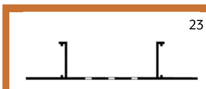
CHANNEL SCREED VENT
